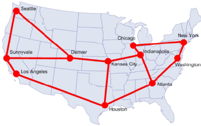
Fig. 2: Experimental setup based on the Abilene backbone topology [14]. Red markers indicate SD-WAN ERs instantiated as Open vSwitches. ERs are connected to Mininet hosts generating probing flows to measure overlay one-way delays.
