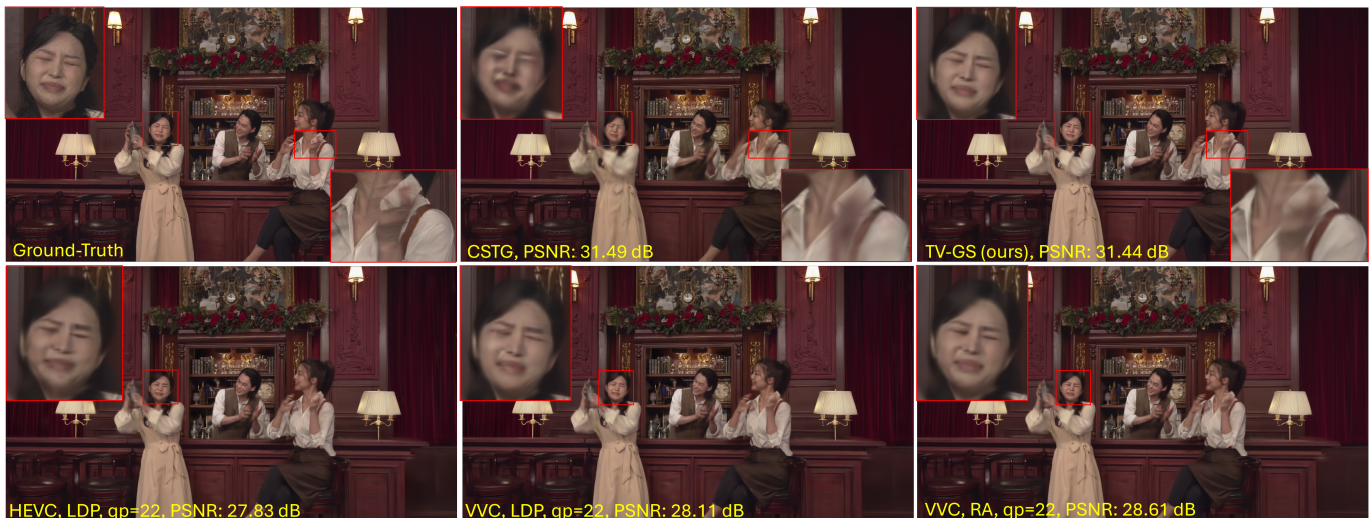
Fig. 3. Visual comparison of rendered test-view on Bartender . Top row : Visual comparison between CSTG and TV-GS. Bottom row : Visual comparison depicting the effectiveness of different video codecs and coding modes on rendering.
