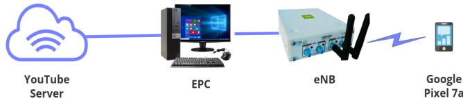
Fig. 1: Realistic LTE testbed with a smartphone
