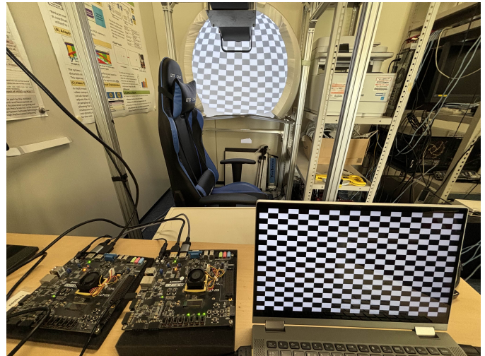
Fig. 2. Projection onto the spherical display after applying the proposed distortion correction. The vertical stretching is successfully eliminated, producing a geometrically faithful image on the spherical surface.
