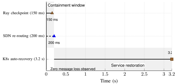
Fig. 6: Recovery timeline: 150–200 ms containment and 3.2 s auto-recovery.
