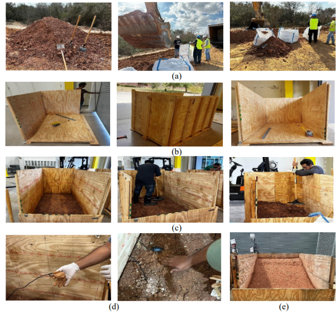
Fig. 2. Physical Slope Model. (a) Soil collection from site; (b) Preparation of wooden box; (c) Soil backfilling, controlled compaction for stability; (d) Installed moisture, temperature, tensiometers sensors at various depths with data logger connected to the sensors for continuous monitoring; (e) Exposed to natural environmental conditions with a weather station installed outside the test section.
