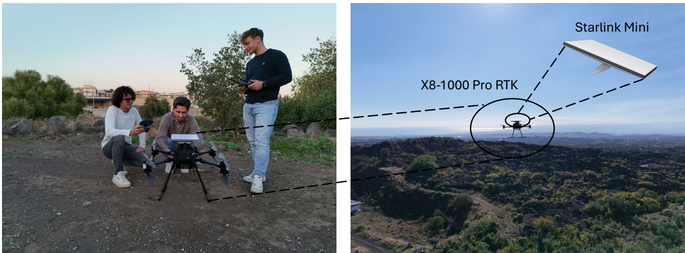
Fig. 2: Some of the authors of the paper with the X8-1000 Pro RTK UAV drone, mounting a Starlink Mini antenna terminal (left). An aerial overview of the experimental rural area near Catania (right).
