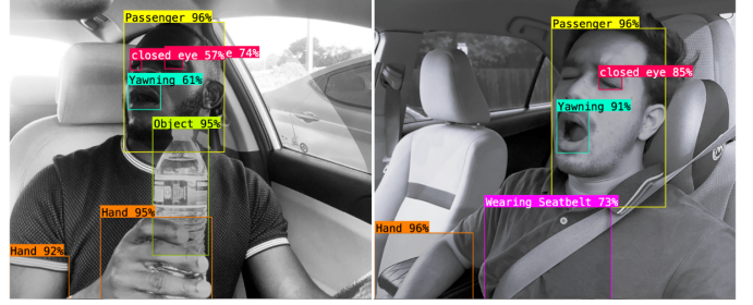
Fig. 5. Representative unsafe driving scenarios. Both drivers exhibit clear indicators of drowsiness, including closed eyes and yawning, reflecting impaired alertness and reduced driving vigilance.
