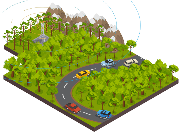
Fig. 1. System Model Visualization. A single-cell 6G scenario where a Base Station serves mobile users moving along a trajectory, subject to dynamic blockage from the environment.
