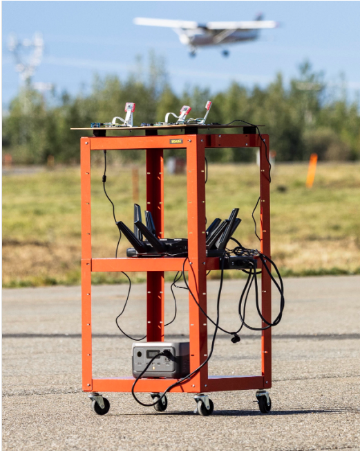
Fig. 4: Sensing pod with passive sensors, edge devices, router, and battery bank.
