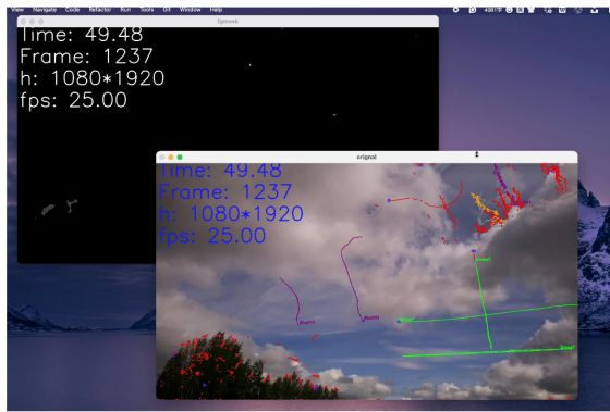
Fig. 6: Sample output of the TRAMIS track-based computation pipeline: object classifications. Here, the classification of multiple UAS and bird tracks within an airspace volume is shown.
