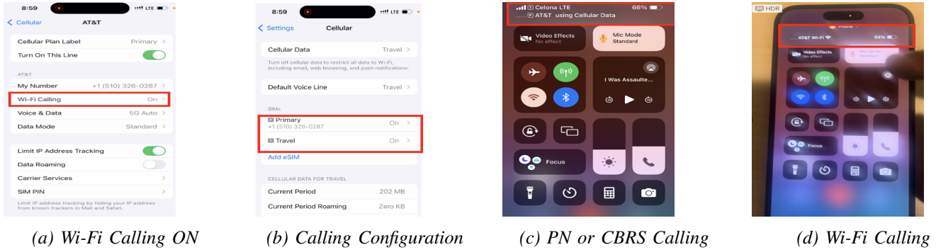
Fig. 4: PN or CBRS and Wi-Fi Calling Configuration
