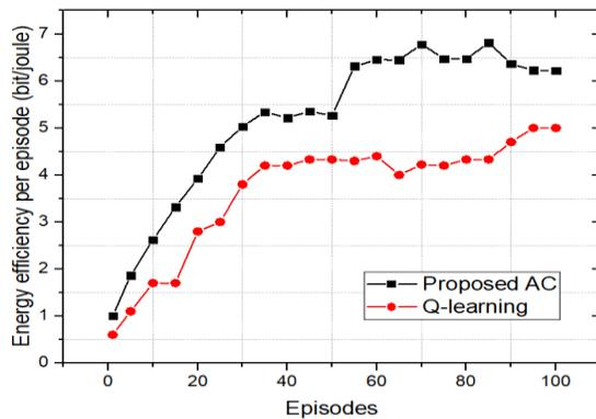
Fig. 2 Energy efficiency comparison with increasing number of episodes.
