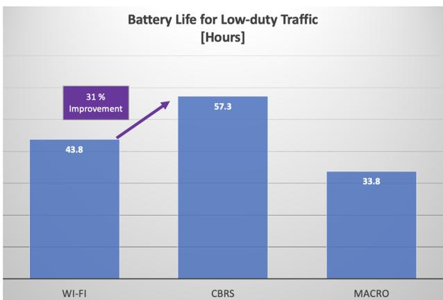
Fig. 5: Static: Battery Life for Low-duty Traffic
