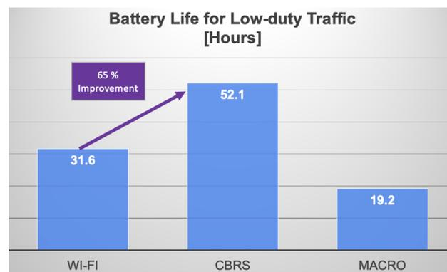
Fig. 7: Mobility: Battery Life for Low-duty Traffic
