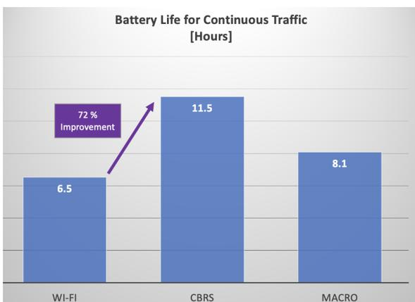
Fig. 4: Static: Battery Life for Continuous Traffic - Zoom
