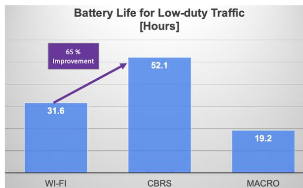
Fig. 7: Mobility: Battery Life for Low-duty Traffic
