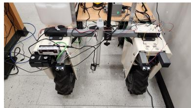
**Fig. 8:** Linear Actuator for Soil Data Aggregation.
