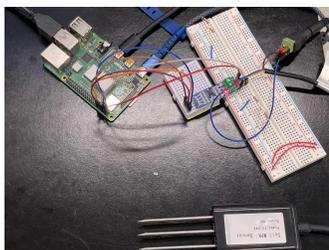
**Fig. 6:** Raspberry Pi to MAX485 to Soil Sensor.
