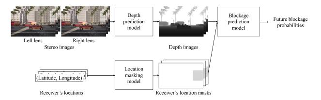
Fig. 1. Proposed blockage prediction system using a stereo camera.
