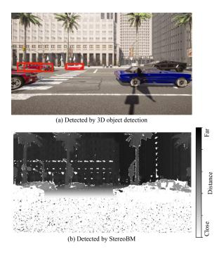
Fig. 5. Examples of blockage features that are used for blockage predictions.
