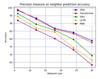
Figure 3: Comparing the precision for different models at predicting their neighbors based off of coordinate data.
