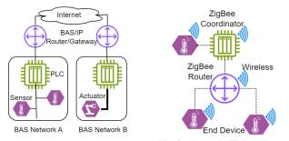
Fig. 2. Example ZigBee Network Fig. 1. Example Wired BAS Network
