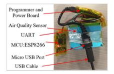
Fig. 5. Inside of the air quality monitoring device
