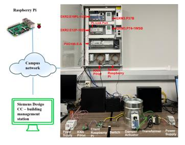
Fig. 6. Smart Building Testbed
