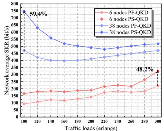
Fig. 3. Performance comparison between PF-QKD and PS-QKD under 6-node and 38-node network topologies.
