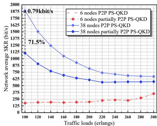
Fig. 5. Performance comparison between PS-QKD and partially P2P PS-QKD under 6-node and 38-node network topologies.
