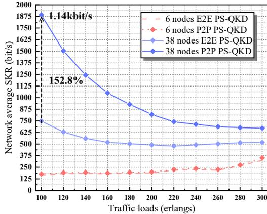
Fig. 4. Performance comparison between E2E PS-QKD and P2P PS-QKD under 6-node and 38-node network topologies.
