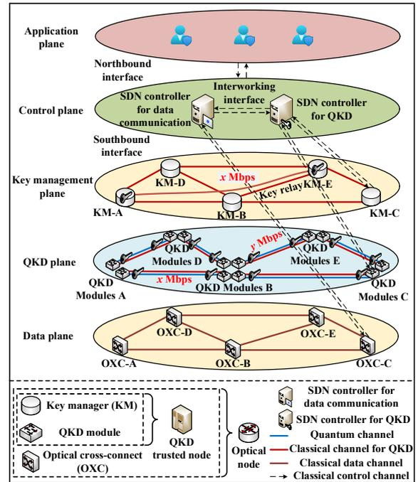
Fig. 1. An optical network architecture for coexistence of classical data communication and QKD.
