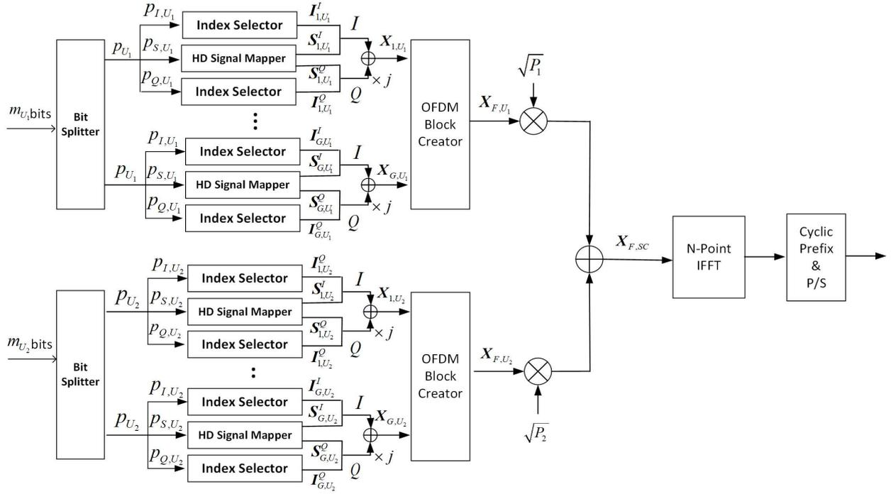
Fig. 1. The structure of HD-IQ-IM-NOMA transmitter.
