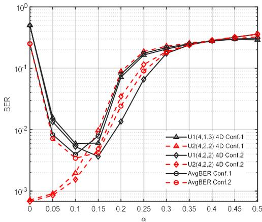
Fig. 3. Optimal  $\alpha$  search from 0 to 0.5 for a fixed SNR of 30dB
