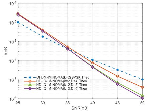
Fig. 2. Theoretical BER curves for individual user under different signal constellations
