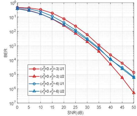
Fig. 5. the BER performance of users under different channel conditions
