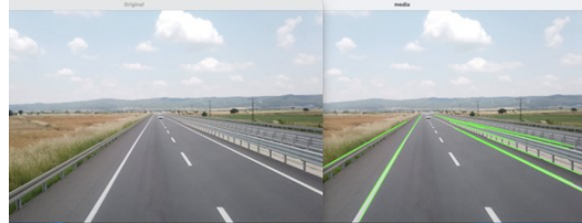
Fig. 4: Hough transform performed on a roadway image original and modified.
