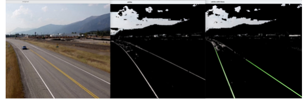
Fig. 5: Color masking and Hough transform performed on a roadway image.
