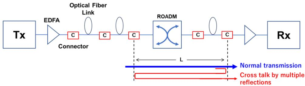
Fig. 2. Optical cross talk noise in photonic network
