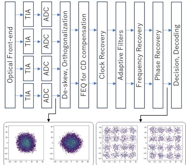
Fig. 3. Block diagram of coherent receiver
