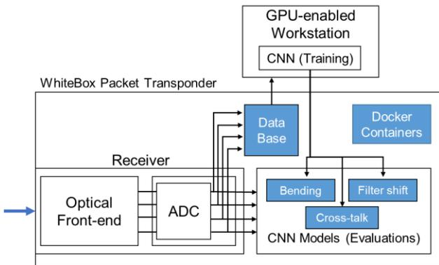
Fig. 5. Sensing system configuration
