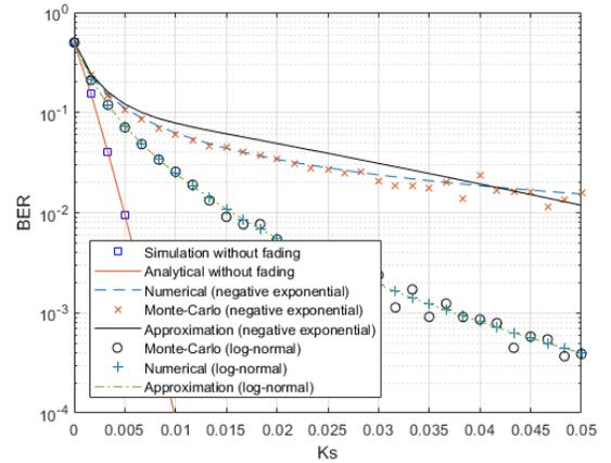
Fig. 4. BER results of SPAD array receiver (64x64) with and without fading channel (log-normal and negative exponential) for values of  $C_{FF} = 0.64$  and  $K_n = 0.001$  ( $T_b = 1\mu s$   $\tau = 1ns$ ).
