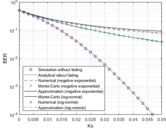
Fig. 2. BER results of SPAD array receiver (64x64) with and without fading channel (log-normal and negative exponential) for values of  $C_{FF} = 0.44$  and  $K_n = 0.05$  ( $T_b = 1\mu s$   $\tau = 1ns$ ).
