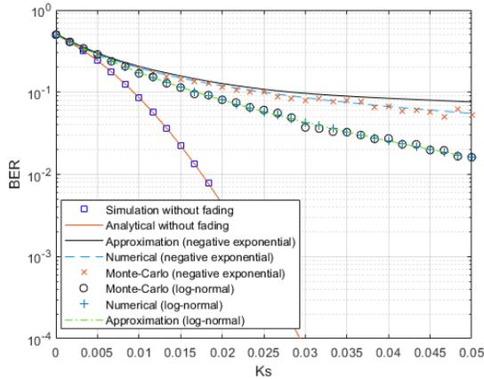
Fig. 3. BER results of SPAD array receiver (64x64) with and without fading channel (log-normal and negative exponential) for values of  $C_{FF} = 1$  and  $K_n = 0.05$  ( $T_b = 1\mu s$   $\tau = 1ns$ ).
