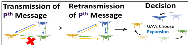
Fig. 3. Example of how UAVs can be resynchronized after Message Loss for the Plume Wrapping Example. With Retransmission , the UAVs do not make a decision till an updated value is received.
