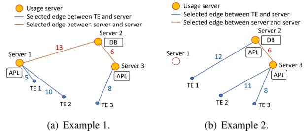
Fig. 2. Example of network configurations. A number attached to each edge indicates the edge delay.
