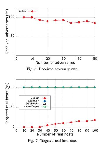
hosts targeted by adversaries is less than 20%. Therefore, we conclude that the proposed model can prevent attackers from targeting real hosts in the network.
