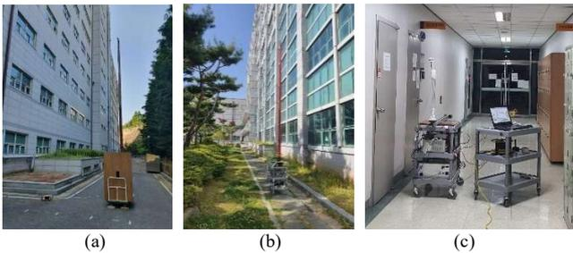
Fig. 3. The measurement setups for building shadowing loss: (a) transmitter (Tx), (b) receiver (Rx) in the opposite, (c) receiver (Rx) with local averaging stage in the corridor
