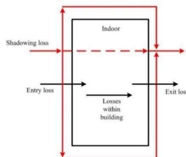
Fig. 1. Schematic view of shadowing loss from Recommendation ITU-R P.2040-1
