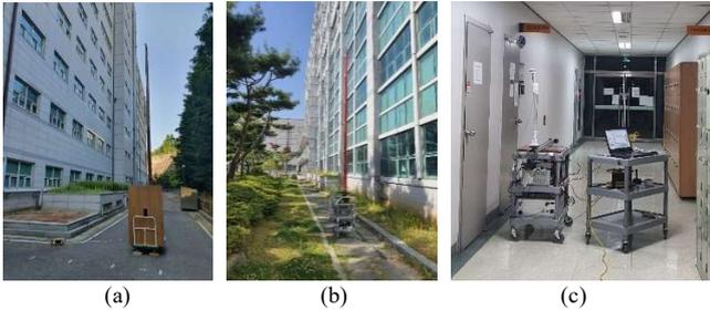
Fig. 3. The measurement setups for building shadowing loss: (a) transmitter (Tx), (b) receiver (Rx) in the opposite, (c) receiver (Rx) with local averaging stage in the corridor
