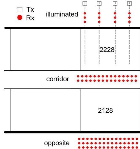
Fig. 4. The Tx and Rx measurement points for building shadowing loss
