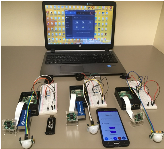
Fig. 6. The Physical Implementation of Smart-Watcher
