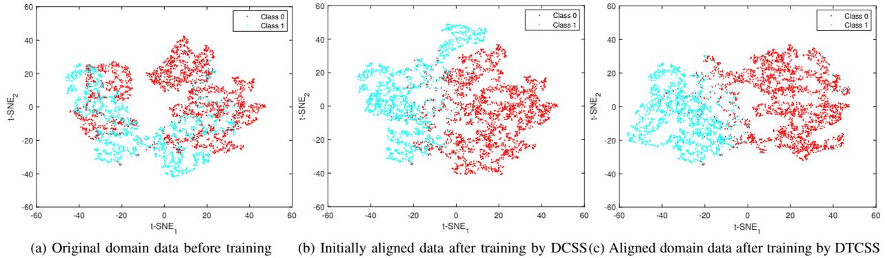
Fig. 3: t-SNE visualization of the source and target domain data at different stages on the transfer task: 16-PSK  $\rightarrow$  Gaussian. For both domains, the red dots in Class 0 means the channel is idle and the blue dots in Class 1 means the channel is busy. The dots with the same color are expected to be aligned.
