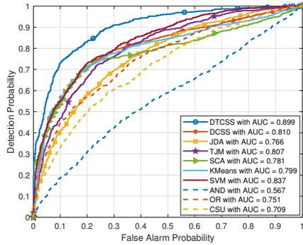
(a) Sensing performance on the transfer task: Gaussian  $\rightarrow$  16-PSK
