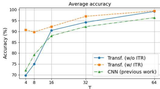
Fig. 6: Average offline accuracy of classifiers for different  $T = \{4, 8, 16, 32, 64\}$ . Performance is compared among transformers with and without the ITR heuristic and CNN model presented in [7].
