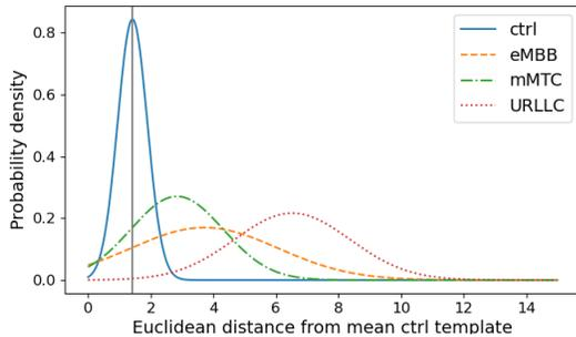
Fig. 3: Visualization of PDF for Euclidean difference for each traffic class ( $T = 16$ ) when compared to mean ctrl template  $\mathcal{T}$ . The solid vertical line is the Euclidean distance value used as the threshold for ctrl relabeling: if the norm of the difference between  $\mathcal{T}$  and an input sample falls below this threshold, the sample is automatically relabeled as ctrl traffic.
