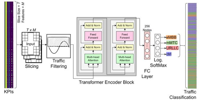
Fig. 1: Transformer-based 5G traffic classification system used in TRACTOR.
