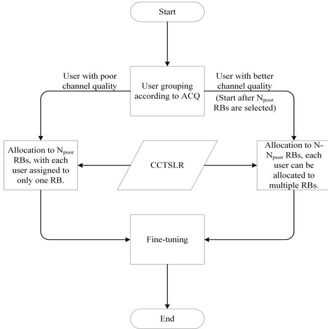
Fig. 2. Proposed resource allocation algorithm
