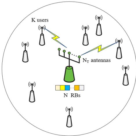
Fig. 1. A single-cell massive MIMO communication system consisting of a  $N_T$ -antennas BS and  $K$  single-antenna users with  $N$  RB resources.
