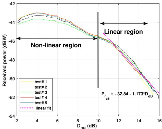
Fig. 5. Received power (dBW) at night versus distance in log domain (dB) for different test cases and expression for linear region with  $K_{dB} = -32.84$  and  $\gamma = 1.173$ .
