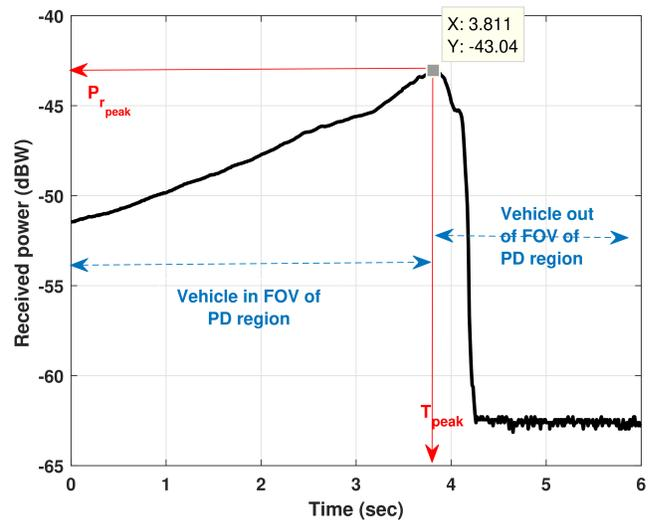
Fig. 4. Received power (dB) at night versus time (sec) with vehicle equipped with normal headlamps.
