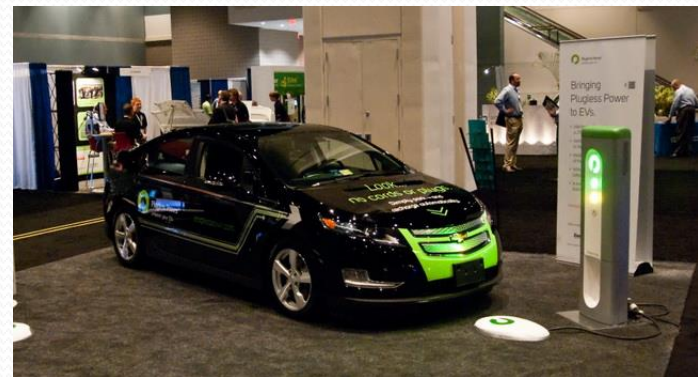
Resonant magnetic coupling charges electrical vehicle.
